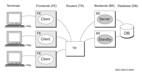
The **transactional shadow server** places all transactions recorded on the primary server on a second database. The transactional shadow server can be at the same site or at a different site, and must exist in a networked environment.
